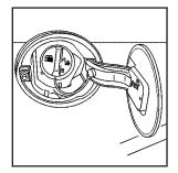
The tethered fuel cap is located behind a hinged fuel door on the passenger side of the vehicle.
